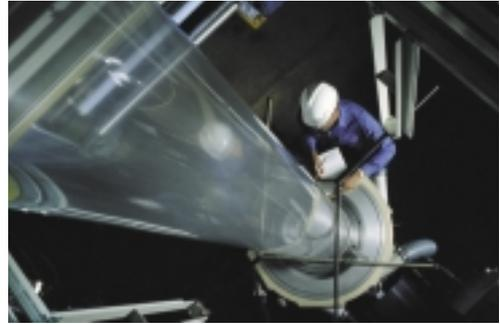
Ongoing temperature measurement of plastics applications such as blown film ensure product quality and productivity. Special models for measuring plastic are available.
